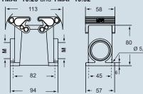
The surface mounting, high construction housings are supplied with an open threaded entry and diametrically opposite a closed threaded entry which can be opened by the user if required (with suitable tool).
