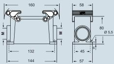
The surface mounting, high construction housings are supplied with an open threaded entry and diametrically opposite a closed threaded entry which can be opened by the user if required (with suitable tool).
